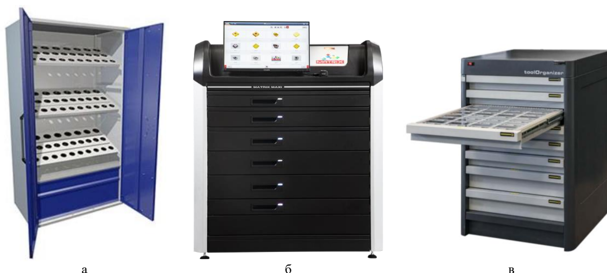
Рис. 1. Типы инструментальных шкафов: а – HARD; б – Matrix Max; в – Zoller tool Organizer Fig. 1. A tool cabinets types: a is HARD; б is Matrix Max; в is Zoller tool Organizer
